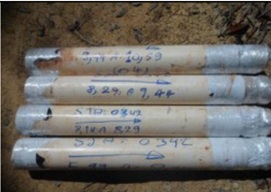
Figure 25 PVC tubes containing core samples (drill hole SJA0342, from Jamari plateau)
