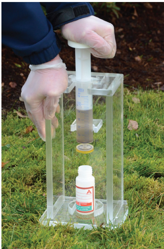
Figure 3. Example of a filtration stand for use in minimizing user contact with the syringe plunger during water filtrations in the field. Image source: “ALS EnviroMail 06 December 2017. Best practices to prevent false positives and negatives for dissolved metals”. Note that vinyl gloves are preferred over nitrile gloves that may host metals contamination.
