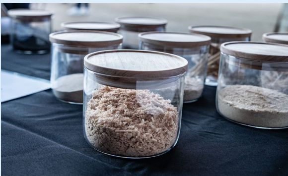
Raw materials for Biolron™ process: biomass, iron ores and fluxes
