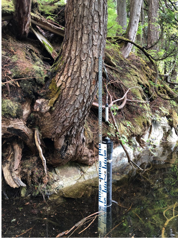
Figure 5. Photo showing the installed water level staff gauge and 2-inch PVC pipe that housed the Hobo water level logger in LAK028.
