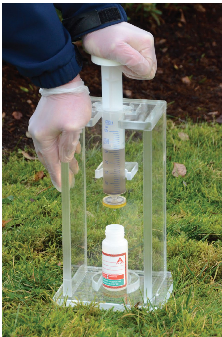
Figure 25. Example of a filtration stand for use in minimizing user contact with the syringe plunger during water filtrations in the field. Image source: “ALS EnviroMail 06 December 2017. Best practices to prevent false positives and negatives for dissolved metals”. Note that vinyl gloves are preferred over nitrile gloves that may host metals contamination.
