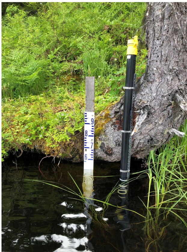
Figure 4. Photo showing the installed water level staff gauge and 2-inch PVC pipe that housed the water level logger in End Lake.
