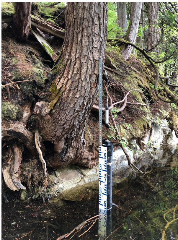
Figure 6. Photo showing the installed water level staff gauge and 2-inch PVC pipe that housed the Hobo water level logger in LAK028.
