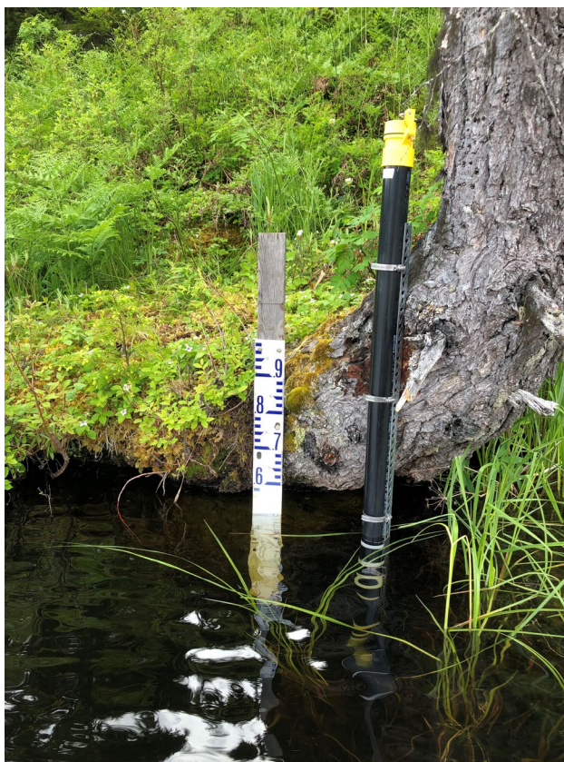
Figure 5. Photo showing the installed water level staff gauge and 2-inch PVC pipe that housed the water level logger in End Lake.
